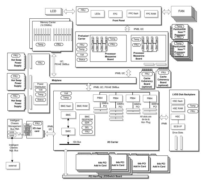
Figure 3-3: OCPRF100 MP Server System Chassis Block Diagram
